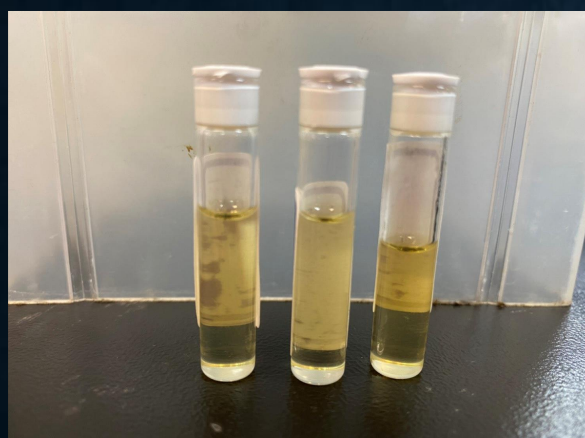
Pic.1 120°C · 0.5g tungstophosphoric acid The ratios from left to right are 1:3, 1:6, 1:9
