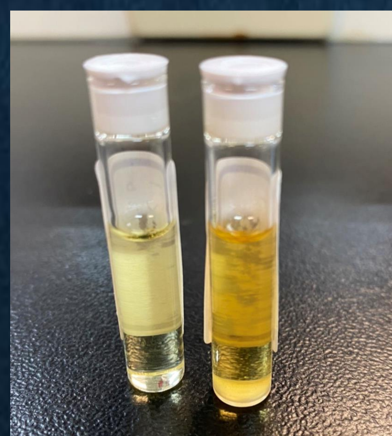
Pic.2 100°C · 0.5g tungstophosphoric acid And 150°C · 0.5g tungstophosphoric acid
